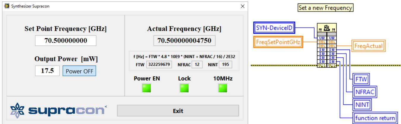
→ There are 6 functions to use the synthesizer. At first you must initialize (Init\_Syn) the synthesizer, then you can work with it (Read\_Syn, Set\_Frequency\_Syn, Set\_Power\_Syn, Switch\_Power\_Syn) and at the end you must close the connection of the synthesizer. Please have a look to program: "Test\_DLL\_Synthesizer.vi".
