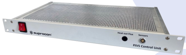
Figure 1. PJVS Control Electronic mounted in a 19-inch-wide one height unit case.
